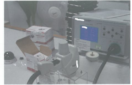
Test device for electrostatic discharge anti-interference
